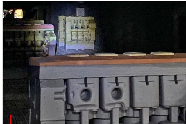
Coated engine block in continuous oven
