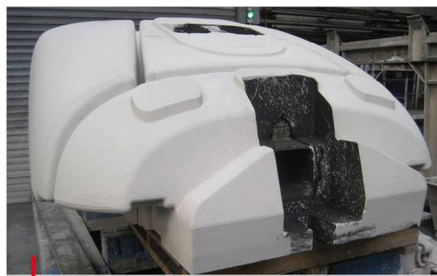
Finished core – 50% faster supplied to moulding line
